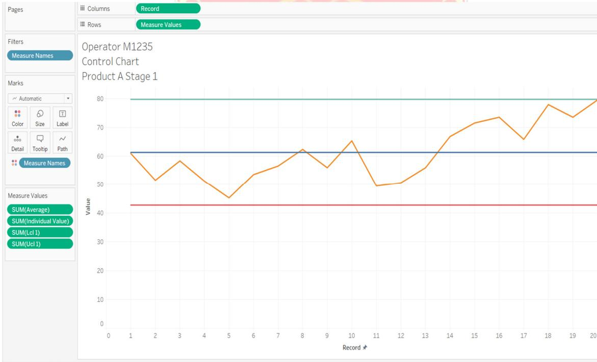
Figure 4: Tableau Visualization of a Moving Range Control Chart for Product A Stage 1 Operator M1235
