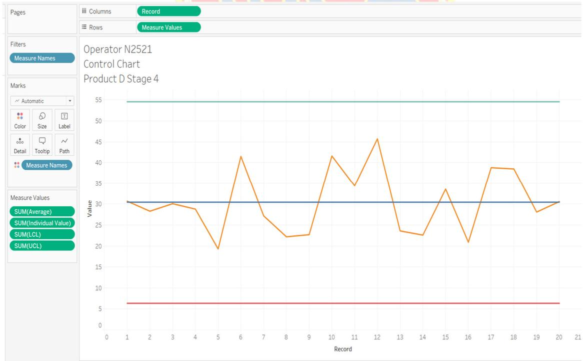
Figure 6: Tableau Visualization of a Moving Range Control Chart for Product D Stage 4 Operator N2521
